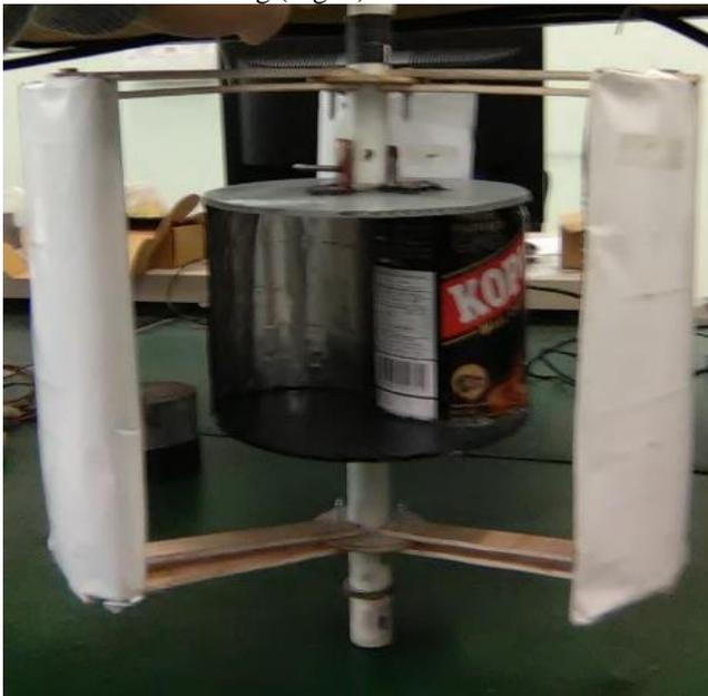
**Fig. 3. Hybrid wind turbine (Savonius - Darrius)**
