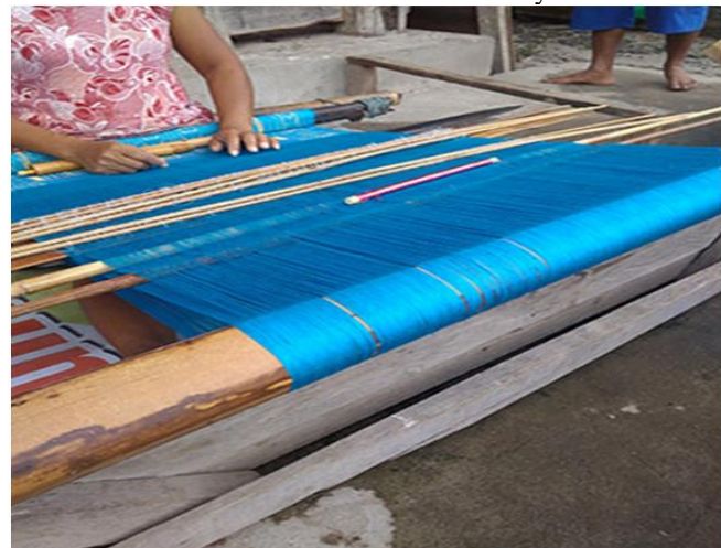
Figure 4.4: (Pangunggasan), for tensing threads
