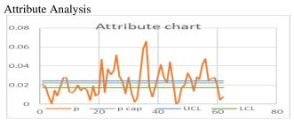
The chart assesses tube rejections compared to their mean, with the p-value exceeding upper and lower control limits (UCL and LCL), indicating outliers with p value 0.221, UCL value 0.024 and LCL 0.017.
