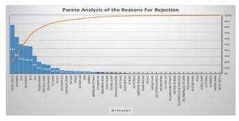
The chart indicates "Short Length" as the top reason for rejection, followed by "ID Scratch" and "Rust," totaling about 60% of rejections.
