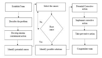
It illustrates identifying the root cause of a problem through a series of steps. The process starts with describing the problem and then establishes a team to address it. If the root cause can't be identified, then corrective actions are taken. If the root cause is found, then potential solutions are identified and corrective actions are implemented. The process concludes with congratulating the team.
